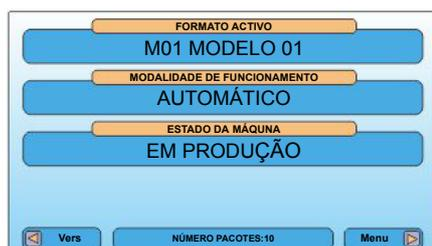
Para parar a máquina, pressionar brevemente a tecla
